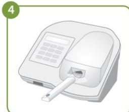
Insert cartridge into RAMP® instrument port. When test is finished, read result.
